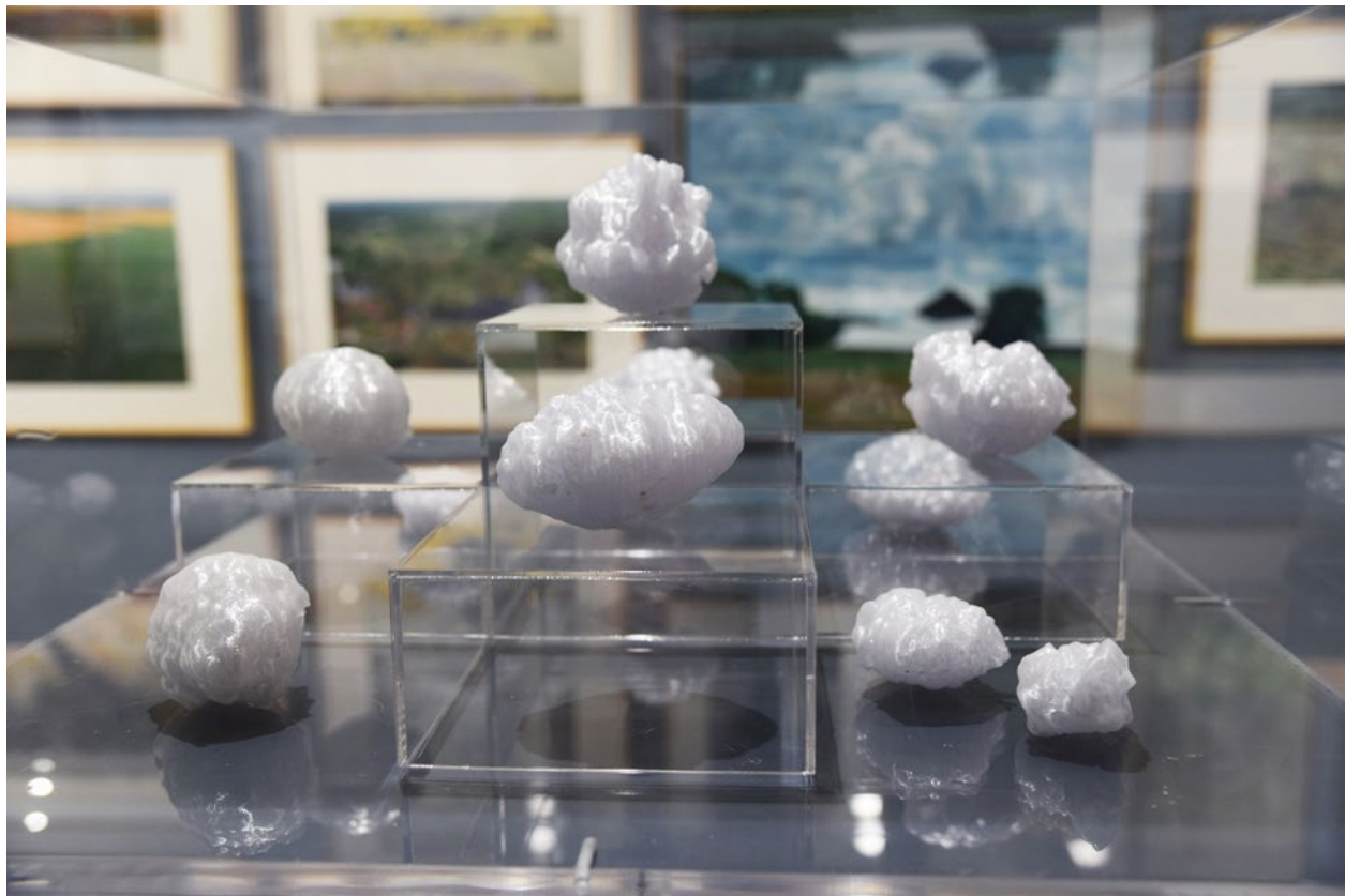
Hailstones, 3D printed with PETG (Polyethylene Terephthalate Glycol) filament at the Canadian Severe Storms Laboratory, Western University.
